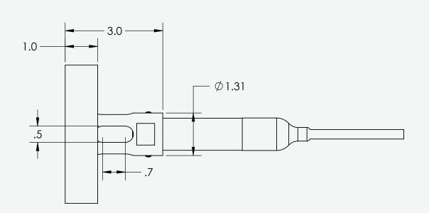
There are many ways to secure your VL2000 Series Depth/Level Transmitter. Popular methods include installing the transmitter in a stilling well, using the optional ½" NPT male conduit connection, attaching the sensor to existing infrastructure, or using a sink weight. Simply connect the VL2000 transmitter to the SW2100 sink weight using the two set screws (included) and drop it into the wet well.
