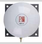
In order to reduce on site maintenance PMC has developed the MP 11 Moisture Protection Reference Volume. For vented gauge transmitters this provides a total isolation to the atmosphere by using a Mylar sphere which changes volume with Barometric pressure. Totally maintenance free. Please specify MP 11.
