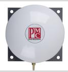
In order to reduce on site maintenance PMC has developed the MP 11 Moisture Protection Reference Volume. For vented gauge transmitters this provides a total isolation to the atmosphere by using a custom bladder while maintaining the high performance of the transmitter. This changes volume with Barometric pressure. Totally maintenance free. Please specify MP 11.
