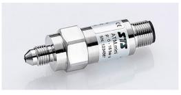
The ATM.mini Pressure Sensor is a high performance sensor, suitable for use in rugged, high vibration environments from -40 to +250°F. The ATM. Mini provides a 2-wire, 4-20 mA or a 3-wire 0.5 - 4.5 Vdc output within a lightweight housing of 0.69" diameter.
