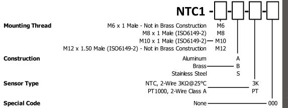
The KA configuration tool is used to specify a standard KA Sensor, other options are available.
