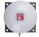
In order to reduce on-site maintenance PMC has developed the MP 11 Moisture Protection Reference Volume. For vented gauge transmitters this provides total isolation from the atmosphere by using a custom bladder, while maintaining the high performance of the transmitter. Totally maintenance free. Please specify MP 11.
