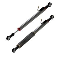
The KP13C compact light duty linear positon sensors are designed to withstand the harsh environments within motorsport and on-vehicle automotive testing applications. By using a proven conductive plastic, track technology and multi-fingered contacts, the KP13C offers high performance and reliability under extreme temperature and vibration.
