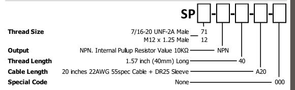
The KA configuration tool is used to specify a standard KA Sensor, other options are available.
