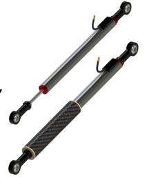
The KP19S standard heavy duty linear position sensors are designed to withstand the harsh environments within motorsport and on-vehicle automotive testing applications. By using a proven conductive plastic, track technology and multi-fingered contacts, the KP19S offers high performance and reliability under extreme temperature and vibration.
