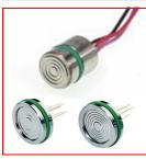
The predominant technology used in the PMC/STS Products is highly developed piezoresistive silicon with repeatability and hysteresis of better than ±0.01%, long term stability of better than 0.05% per year, and operating range of -40 to 300°F
