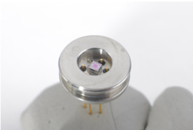
The silicon sensor element inside the glass-to-metal seal
